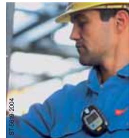
Figure 1: Gas detector Dräger Pac 5000 carried by personnel
